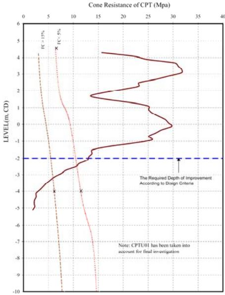
Fig. 6. Results of  $q_{c,Post}$  for segment R1C
