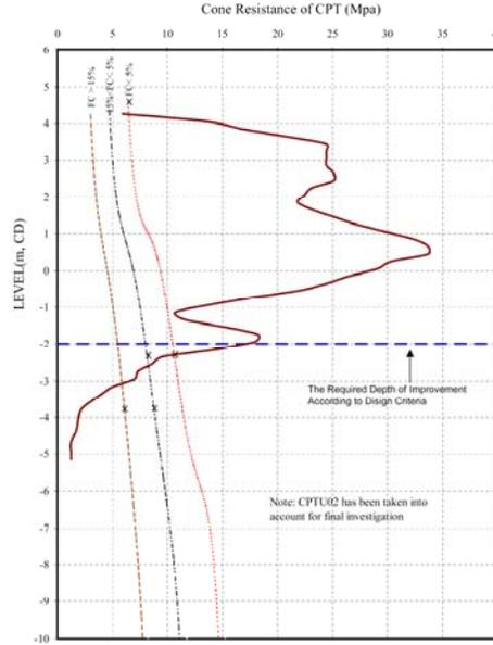
Fig. 7. Results of  $q_{c,Post}$  for segment R2D
