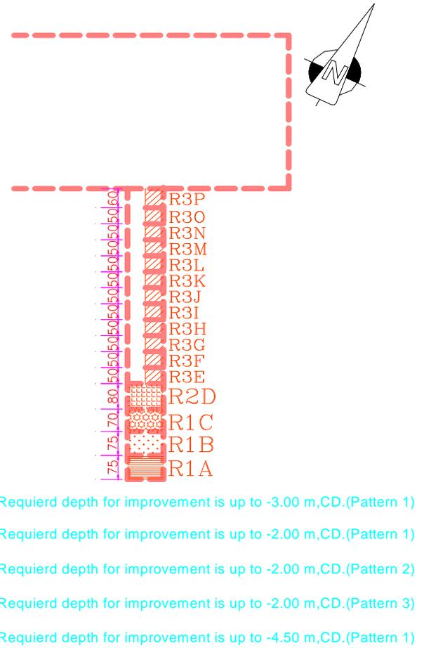
Fig. 5. Improvement segments for the eastern region behind the quay walls
