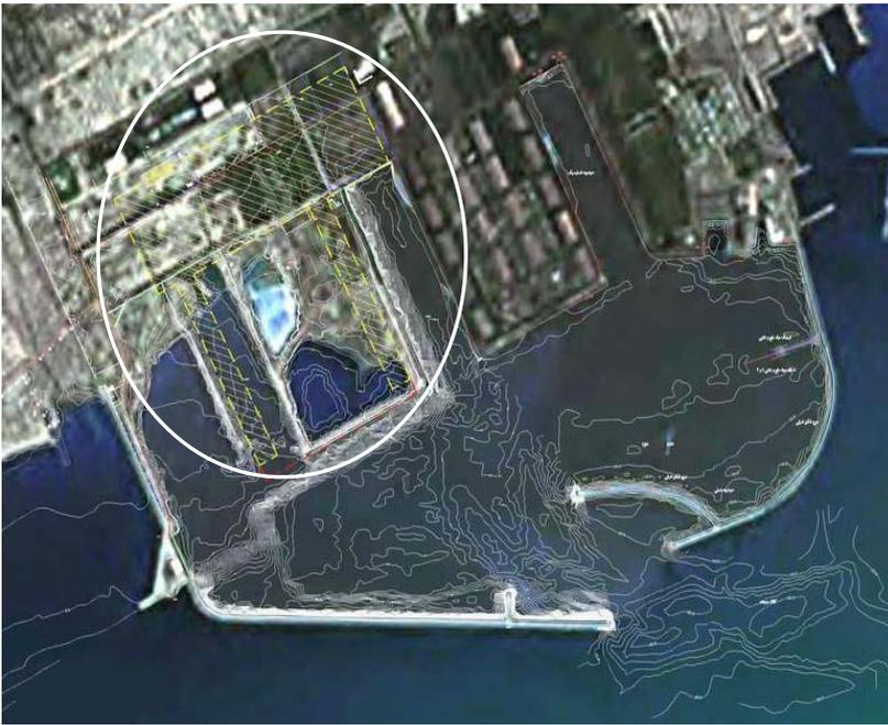
Fig.1. Plan of the S.R.P.C.D. Stage 2 project: 2 western and eastern container berths and northern stacking yard
